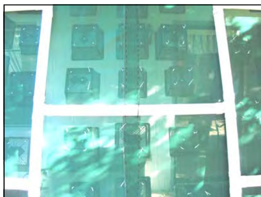
Bottom view of baskets wire tied to trampoline
